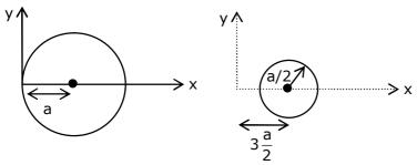
$$X_{com} = \frac{(\sigma \times \pi a^2 \times a) - (\sigma \frac{\pi a^2}{4} \times \frac{3a}{2})}{\sigma \pi a^2 - \frac{\sigma \pi a^2}{4}}$$
